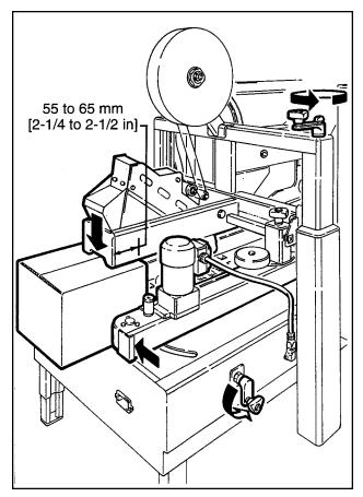
Figure 3-7 – Box Size Set-Up
